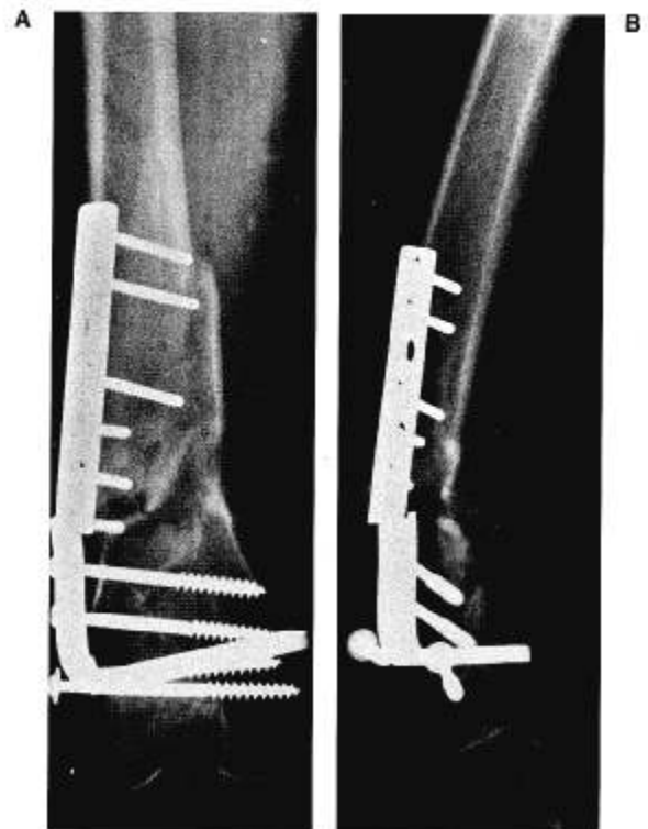
FIG. 2. (A) AP and (B) lateral radiographs showing fatigue fracture of the blade plate at 4 months with more anatomic alignment of distal femur.
